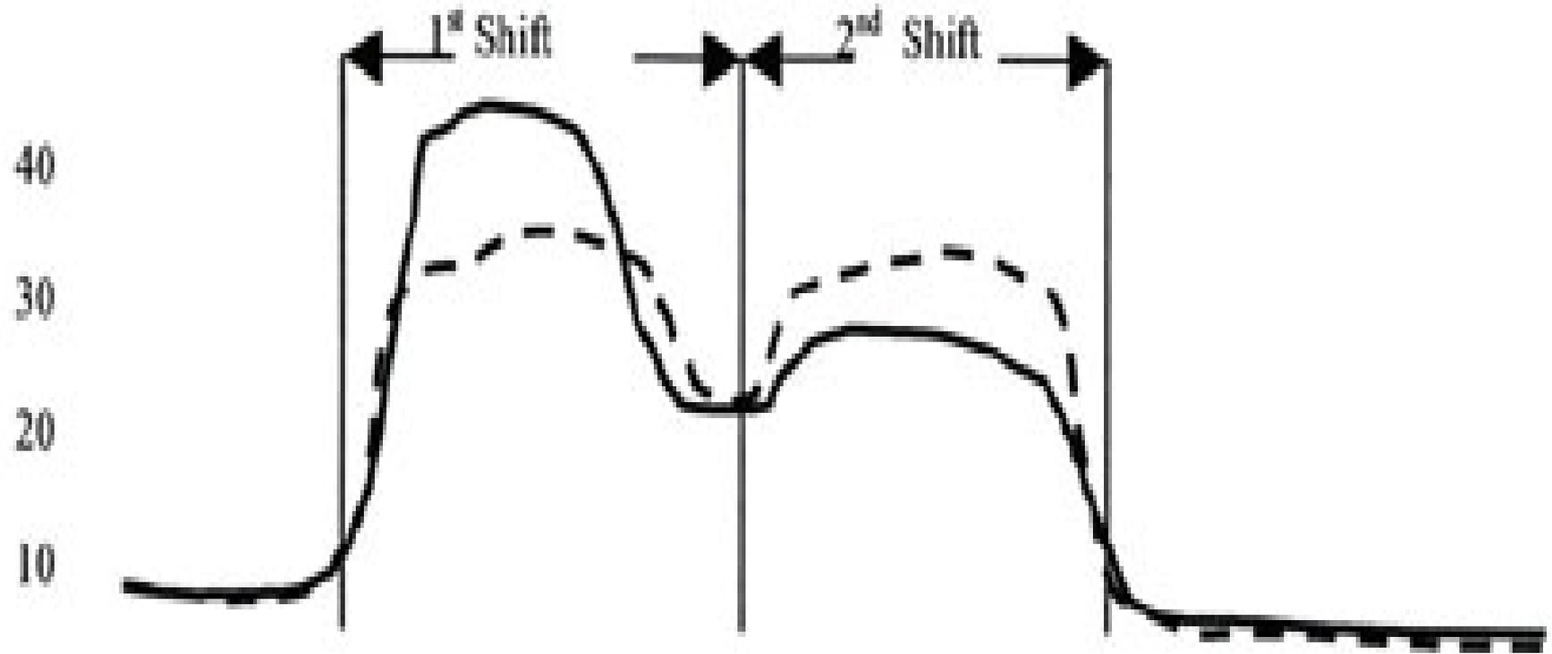
Solid line represents normal demand profile. Dotted line represents lower demand profile that can be obtained by shifting a portion of the electric load from the first shift to the second shift.
