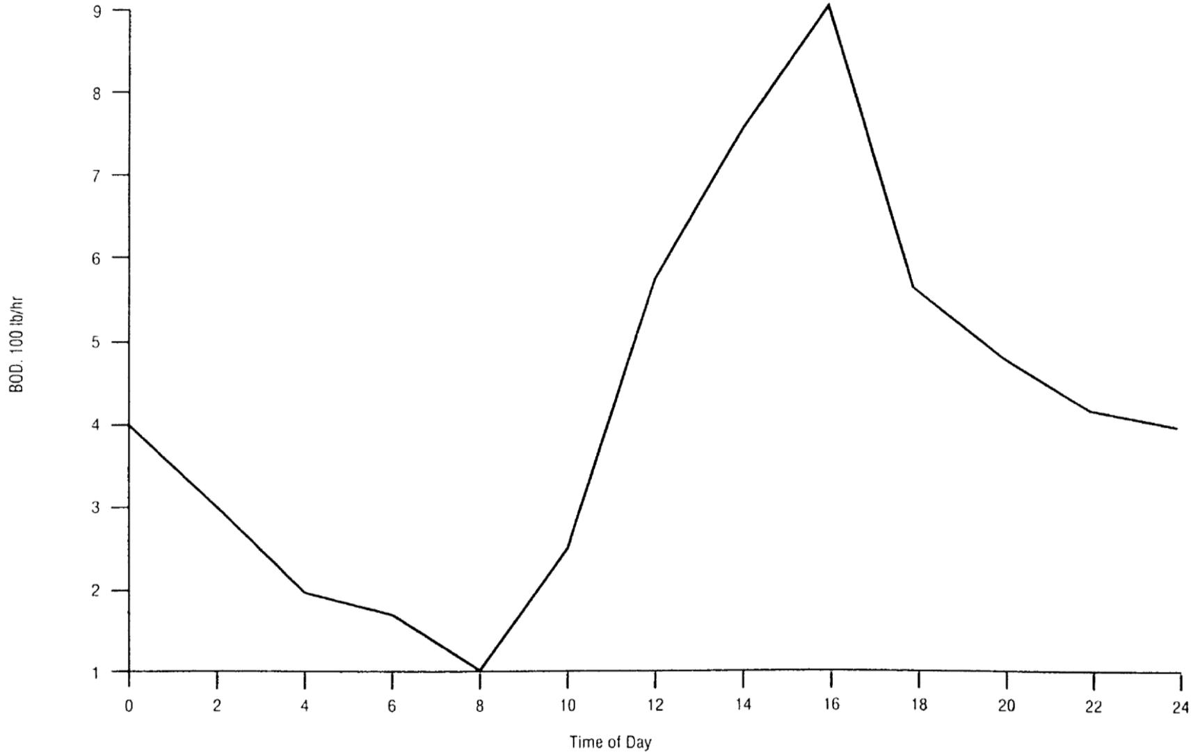
Figure 2. Variation in influent wastewater strength over 24 hours for a typical treatment plant.
